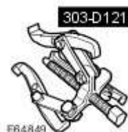
Remover, crankshaft seal 303-D121
