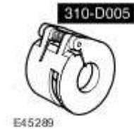
Fuel spring lock decoupling tool 310-D005
