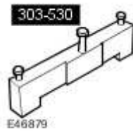
Camshaft setting/locking tool 303-530
